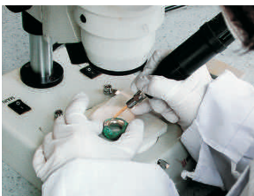
Cleaning: Remove dirt and rust as much as possible with the highest caution of not to damage the items
